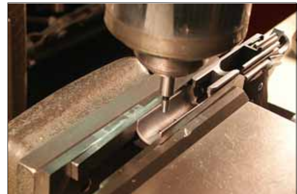
Step 11: Zero From Inside Of Frame, And Then Center On \frac{1}{2} The Width Of The Dust Cover Interior, Roughly .630" On Most Models.
