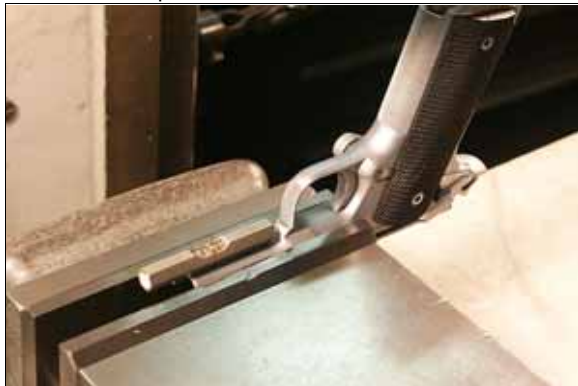
Step 2: Chuck Frame In Vise And Level. Use Very Little Pressure To Avoid Frame Crush.
