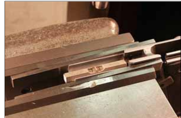
Step 10: Clamp Frame Right Side Up In Vise And Level. Use Very Little Pressure To Avoid Frame Crush.
