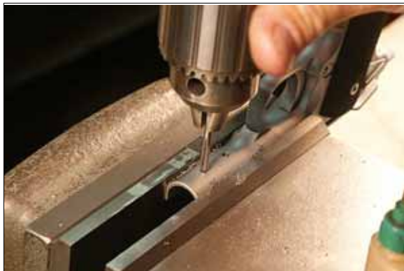
Step 8: Tap Both Holes 6-48. Lubricate While Tapping.
