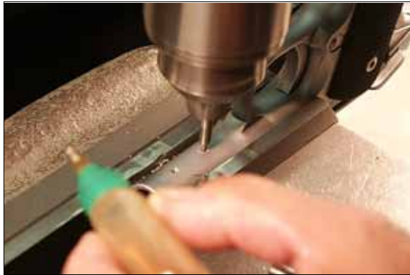
Step 6: Drill Second Starter Hole .670" From The First Hole, or 1.235" From End Of Dust Cover. Lubricate While Drilling.
