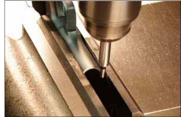
Step 3: Zero Front-To-Back On Inside Surface Of Vise, And Move To Center. Center Is 1/2 Width Of Dust Cover, or Roughly .750" For Most Models.
