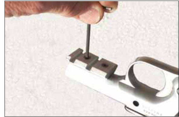
Step 9: Install Rail On Dust Cover With 6-48 Screws Provided. Use Blue Lock-Tite Only. Wipe any excess Lock-Tite Out Of The Dust Cover.
