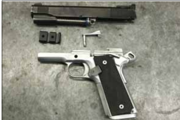
Step 1: Remove Slide From Frame.
